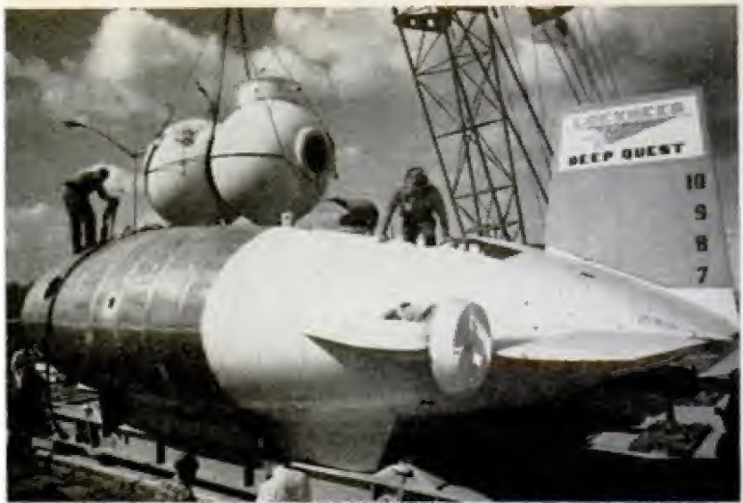
MARAGING STEEL , a specially processed nickel-alloy steel, gives added strength to the twin pressure hulls of Lockheed's Deep Quest
